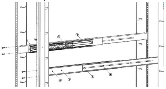
**Step 2:** Slide shelf into rack by aligning the detached inner slide with the installed outer slides and sliding the shelf all the way in.
