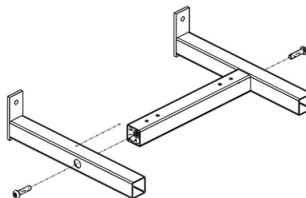
Note: The channel nut teeth should always face towards the bolt head.
